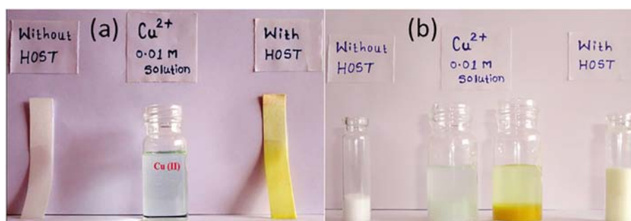
Fig. 7. Practical application of PP3 to detect \text{Cu}^{2+} by: (a) test strip and (b) Solid support techniques.
