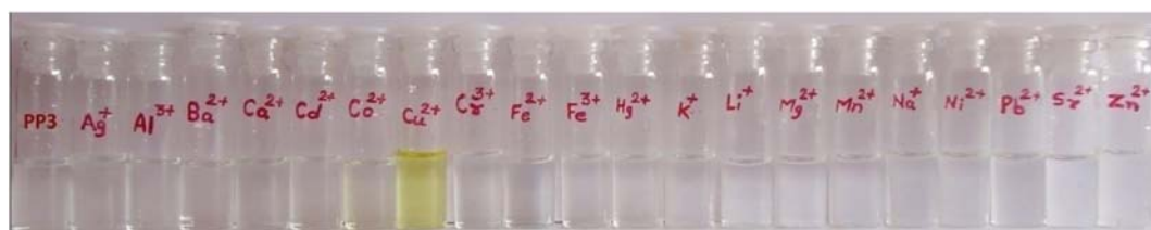
Fig. 1. Naked-eye recognition of \text{Cu}^{2+} : the vials containing PP3 (2 mL, 1.0 \times 10^{-3} M) in EtOH: \text{H}_2\text{O} (20:80, v/v) upon addition of various metal ions (1 mL, 1.0 \times 10^{-2} M, in \text{H}_2\text{O} ).
