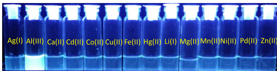
Fig. 1. Vials irradiated with UV light at 365 nm containing BPB (2 mL, 1 \times 10^{-5} M, in CH 3 OH) in presence of ~5 equivalents ( 4.76 \times 10^{-5} M) of different tested metal ions (100 \mu\text{L} , 1 \times 10^{-3} M, in H 2 O).
